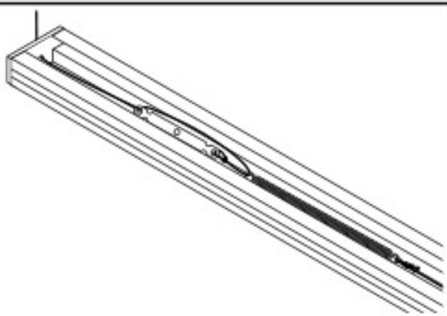
Gently remove the insert from the channel in the bottomrail, revealing the spring tension components. Keep insert. Remove tape securing the components.
