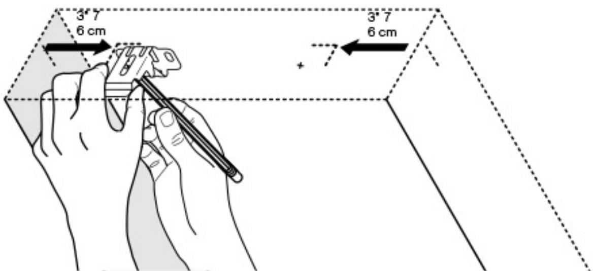
Measure in 3" from the marks made in step 3. Hold brackets up to the marks and mark screw locations using top hole of bracket. For shades over 42", mark center for third bracket.
