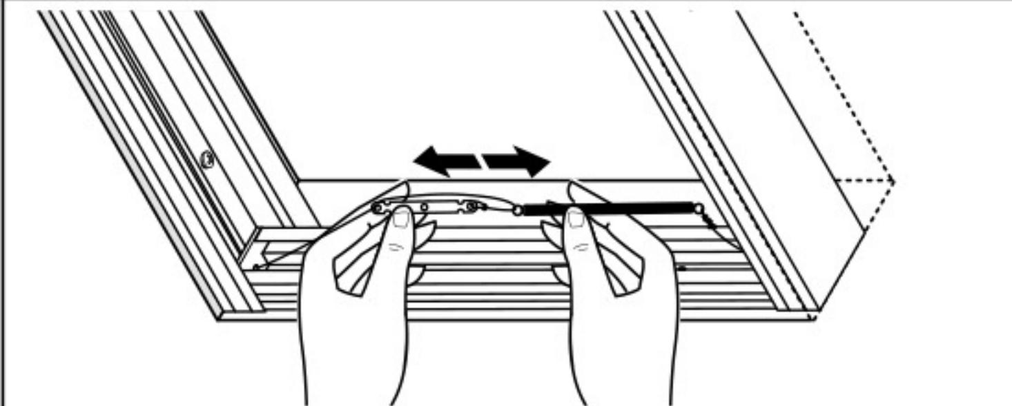
Remove the tie holding the shade and check the cord tension. If the tension is too loose, move the tension plate in the bottomrail away from the spring. If it is too tight, move the tension plate toward the spring.
