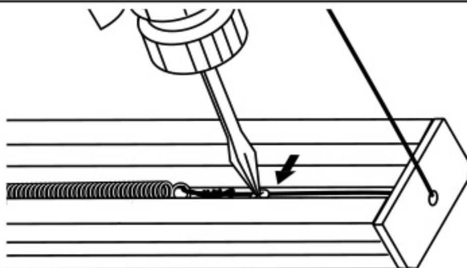
Loosen screw closest to the spring. Place cord under the screw head and tighten.
